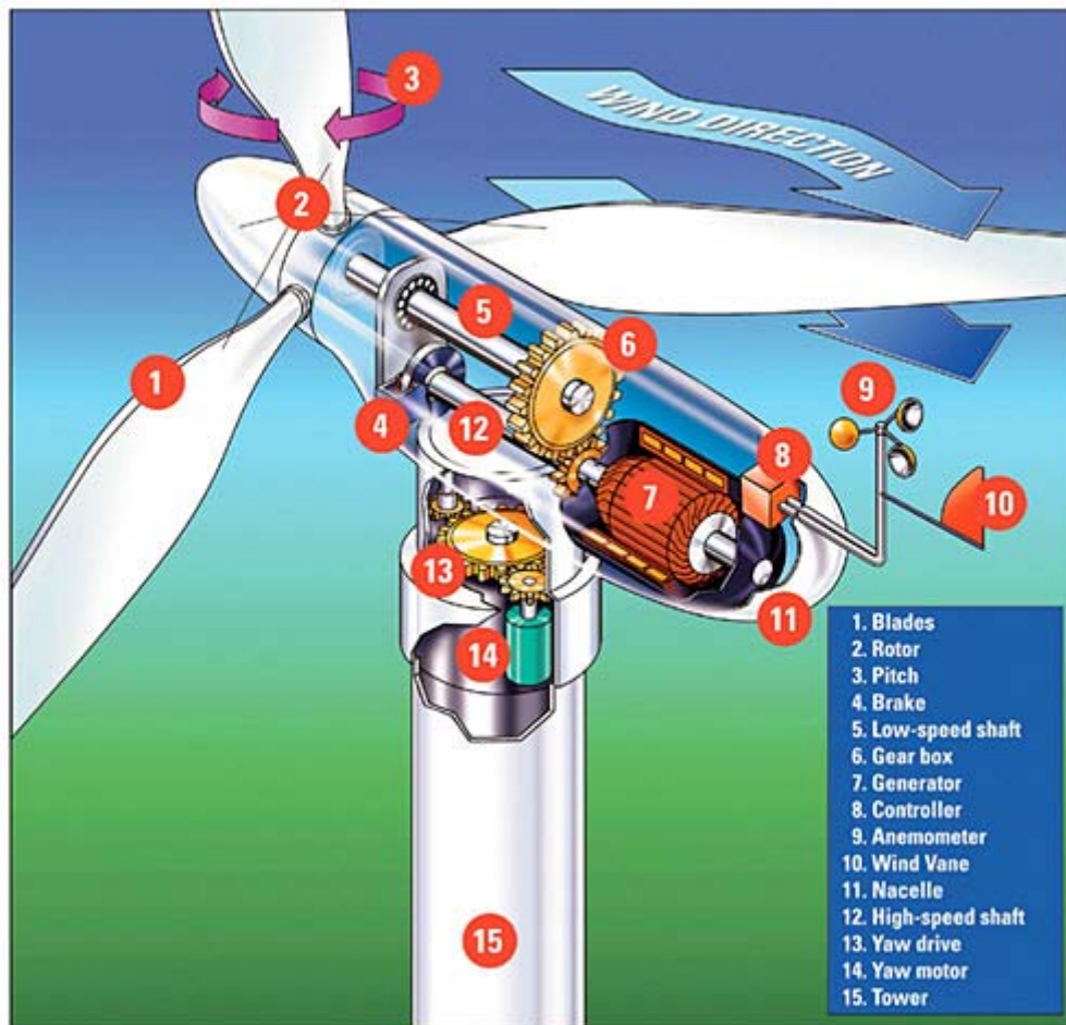
A diagram of the parts to a wind turbine
