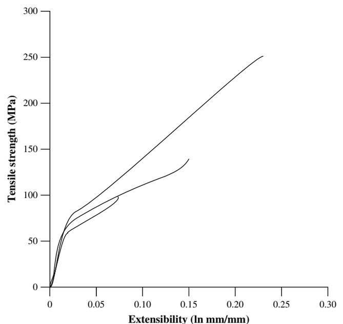
Fig. 3. Three representative stress–strain curves of *Antipaluria* silk tensile tests that depict the maximum, median, and minimum true stress values.
