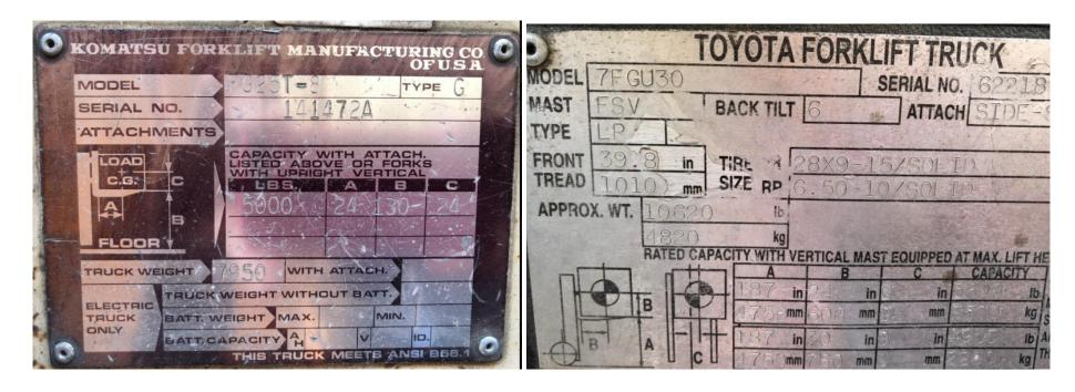
Plates are required to be on Powered Industrial Trucks. Do not lift items above the rated capacity.
