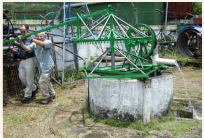
Ahmed Amer and Jim Reites, S.J., operate a rope pump system in Nicaragua.
