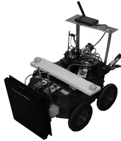
Fig. 4. Experiment utilized Pioneer robots with custom communication and force sensing equipment. One of the two robots used is shown above.
